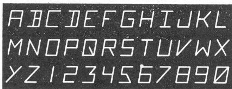
Fig. 2—Above are the cathode segments that are used to display both numbers and alphabet letters.
