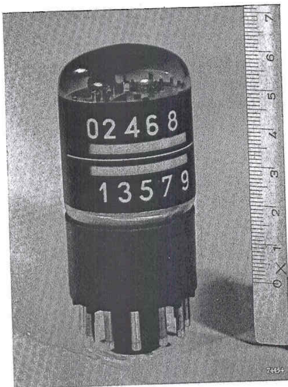
Fig. 1. The EIT decade counter tube. A blue fluorescent mark indicates the figure which corresponds to the position of the electron beam in the counter tube, i.e. to the number of pulses counted.
