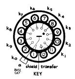
The G10/241E is a single-ended cold-cathode unidirectional gas-filled counter and distributor tube. It has ten cathodes which are used to indicate the number of the count, either visually at low speeds or by means of the voltage developed across the cathode load at high speeds. It is capable of counting pulses at repetition speeds from approximately 0 up to 20 kc/s.
