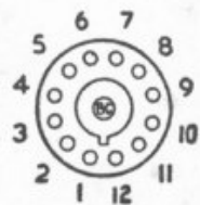
Base Connections (underside view)
