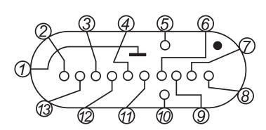
Pin numbering starts clockwise from the first pin, which is labeled on the component capsule by an arrow. The pin numbering scheme above is valid when the component is observed from the bottom.
