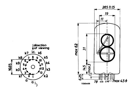
1) Pins 1 and 2 to be interconnected externally.
