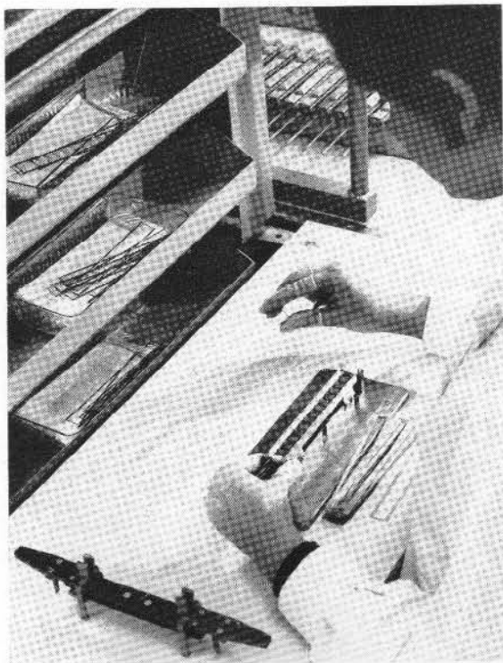
Fig. 2. A Jacob's ladder worked by a foot switch presents numerical cathodes to the assembler in the order in which they are to be fitted over the anodes. Mica insulating frames (alongside the assembly jig) are placed between each pair of electrodes.
