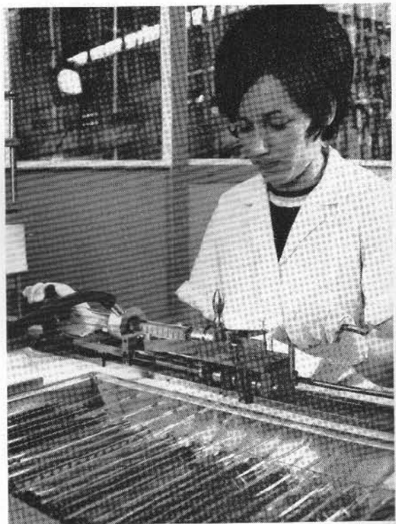
Fig. 5. A fixture guides the electrode and base assembly into the glass envelope. Air blown in at the far end of the envelope sweeps detrital flakes of mica towards the entry for extraction by an annular suction nozzle.
