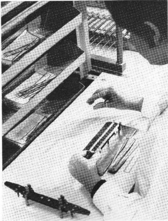
Fig. 2. A Jacob's ladder worked by a foot switch presents numerical cathodes to the assembler in the order in which they are to be fitted over the anodes. Mica insulating frames (alongside the assembly jig) are placed between each pair of electrodes.
