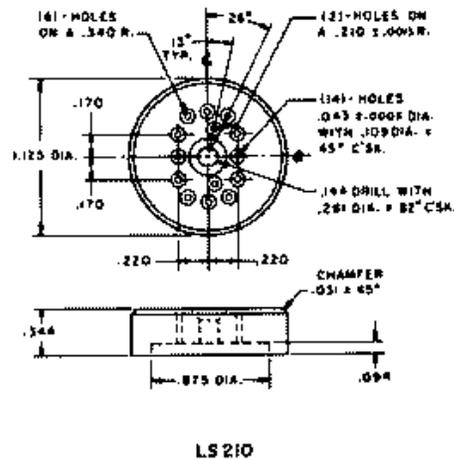
Figure 6. PIN STRAIGHTENERS
